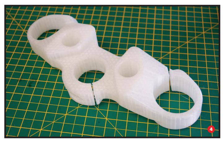
If you get that right, you start the build, have the machine pause where you need it to, remove the build plate from the machine, add your hardware, then snap it back into place and complete the job.
